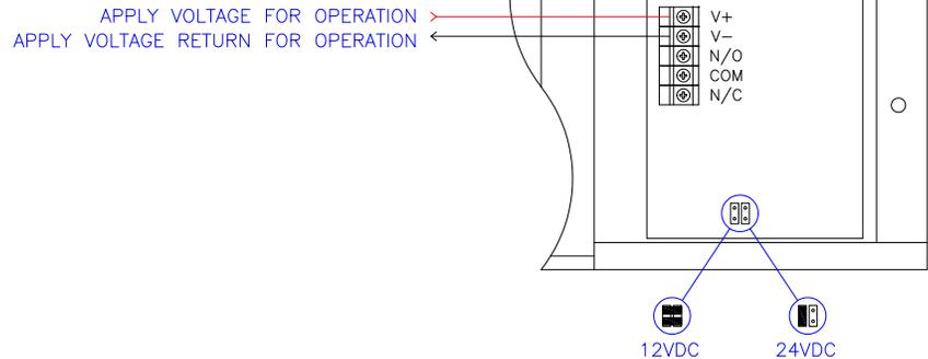
INSTALL JUMPER TO SOURCE 12VDC JP1
